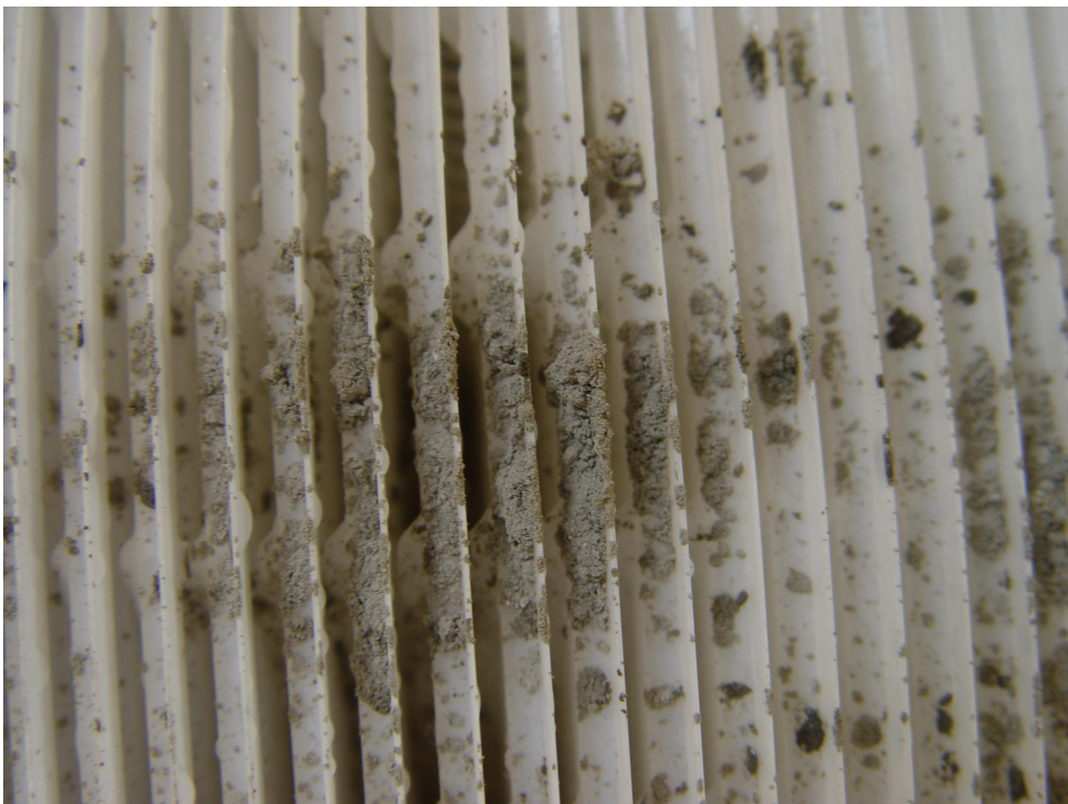
Figure 2: "RS 160" heat exchanger after contamination, before cleaning
