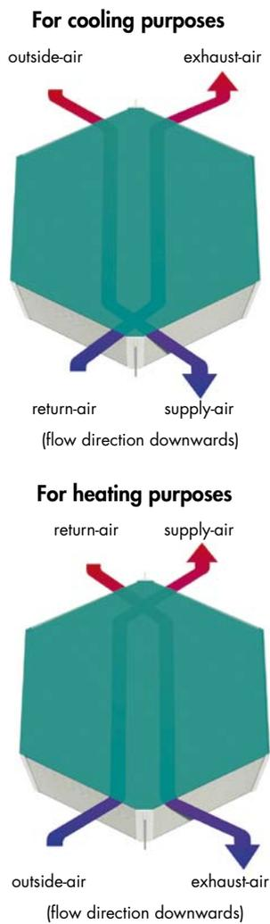
Figure 8: Mounting orientation "on the (white) side panels"
